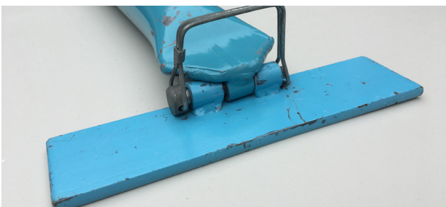
Figure 5. Pin with safety snap securing the end of new blow pipe.
